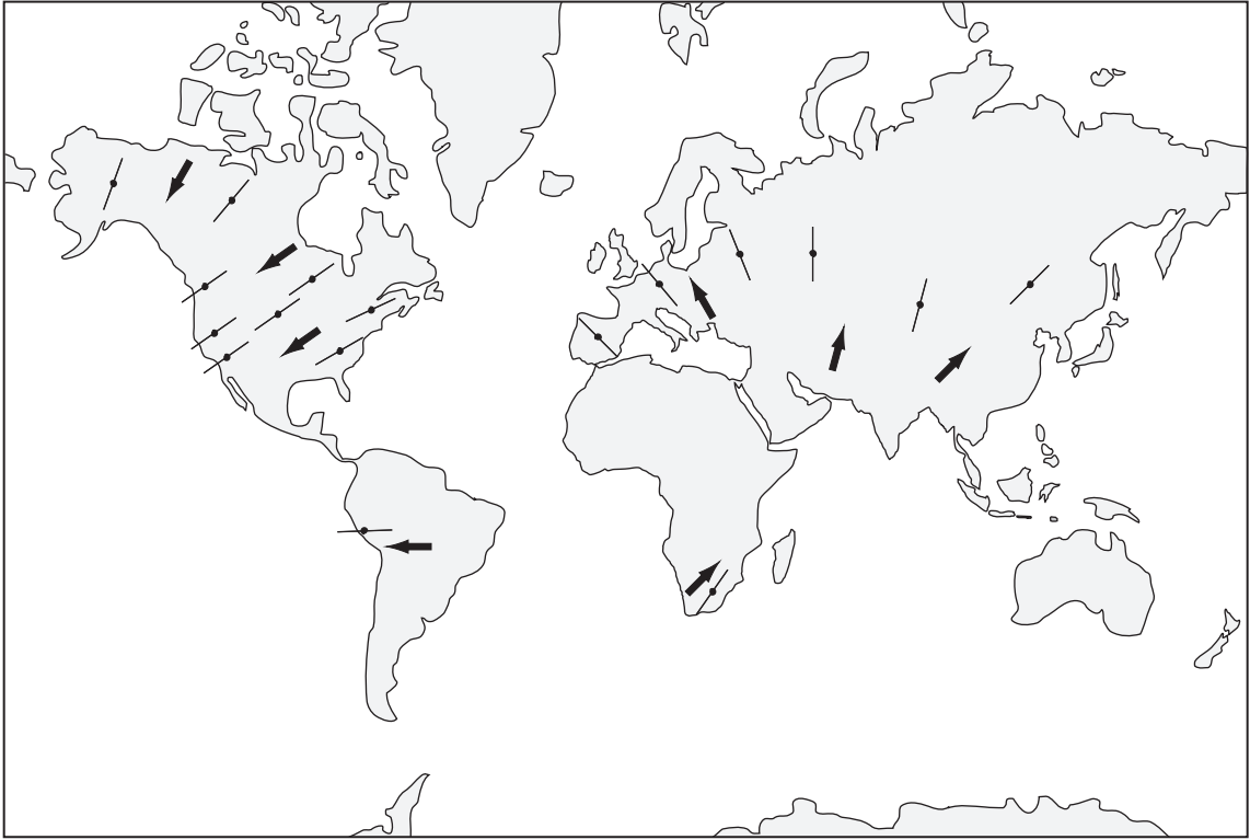
Figure 4.12 Fast S-wave velocity directions in the subcontinental lithosphere compared with motion directions of modern plates (bold arrows). Modified from Silver and Chan (1991).
